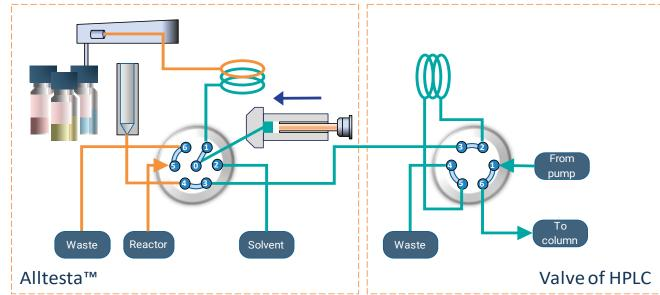
8 Excess of sample to a vial. Extra solvent for controlled dilution.
