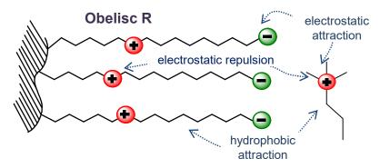
Figure 3. Different types of interactions of quaternary amines with Mixed-Mode columns
