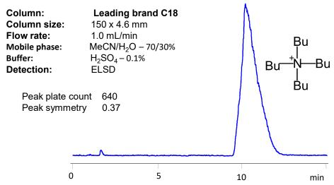
Figure 2. Retention of Tetrabutylammonium on RP column
