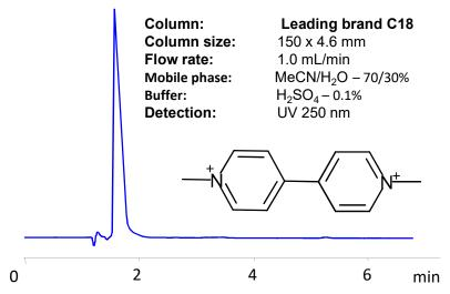
Figure 1. Retention of Paraquat on RP column
