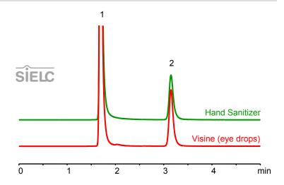
Fig. 3. Isocratic chromatogram of EDTA complex with Fe(III). HPLC column: Newcrom BH, 4.6 x 150 mm, 5  $\mu$ m. Flow rate: 1.0 mL/min. Mobile phase: 2% MeCN in water containing 0.1%  $H_2SO_4$ . Detection: UV 260 nm.
