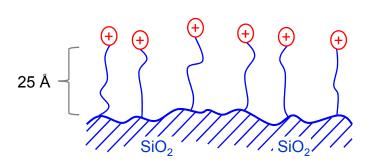
Fig. 6. Schematic structure of Newcrom BH column surface chemistry
