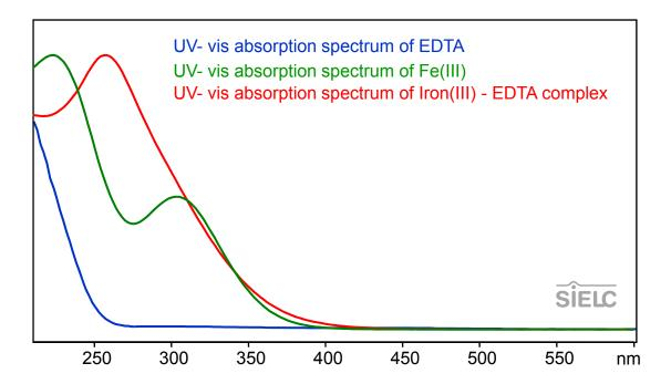
Fig. 1. UV spectra of EDTA • Fe(III) complex, FeCl<sub>3</sub> solution, and EDTA solution.
