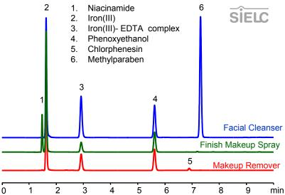
Fig. 4. Gradient method. HPLC column: Newcrom BH, 4.6 x 150 mm, 5  $\mu$ m. Flow rate: 1.0 mL/min. Mobile phase: MeCN gradient from 2 to 70% in water in 10 min, mobile phase contains 0.1%  $H_2SO_4$ . Detection: UV 260 nm. Injection: 5  $\mu$ L of sample.
