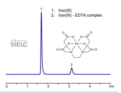
Fig. 2. Chromatogram of EDTA complex with Fe(III). HPLC column: Newcrom BH, 4.6 x 150 mm, 5  $\mu$ m. Flow rate: 1.0 mL/min. Mobile phase: 2% MeCN in water containing 0.1%  $H_2SO_4$ . Detection: UV 260 nm.
