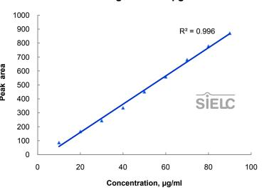
Fig. 5. Linearity study of the EDTA analysis quantitation method. Analytical column: Newcrom BH, 4.6 x 150 mm, 5  $\mu$ m. Flow rate: 1.0 mL/min. Mobile phase: 2% MeCN in water containing 0.1%  $H_2SO_4$ . Detection: UV 260 nm. Injection: 5  $\mu$ L of EDTA standards with FeCl<sub>3</sub> solution.
